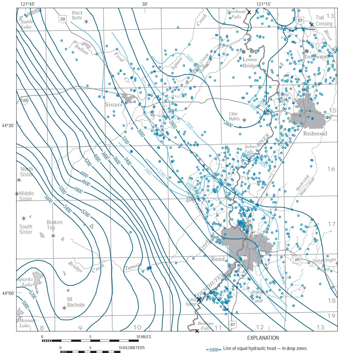
**Figure 30.** Generalized lines of equal hydraulic head for shallow and deep water-bearing zones in the central part of the upper Deschutes Basin, Oregon. (Elevated heads in shallow zones are due to infiltration of water from leaking irrigation canals, on-farm losses, and stream leakage.)
