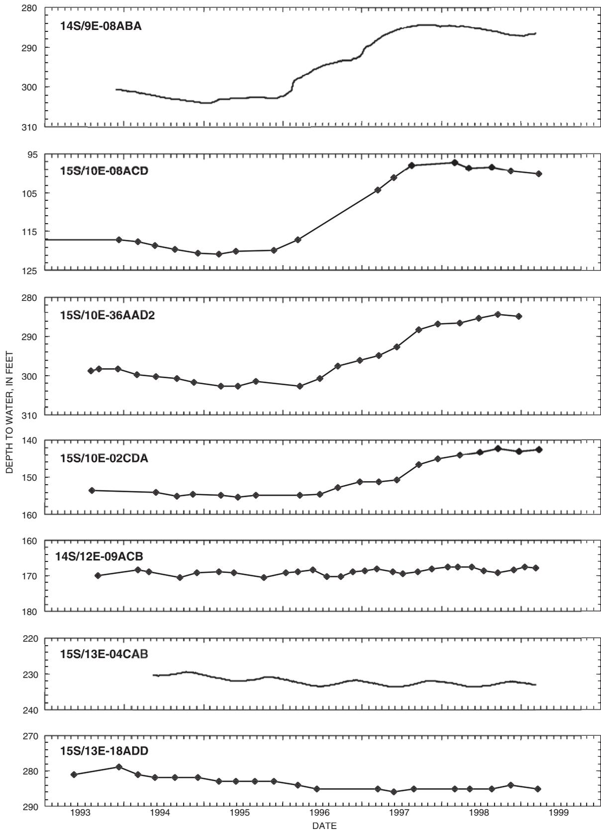
**Figure 32.** Variations in static water levels of selected wells at various distances from the Cascade Range, 1994–98. (The hydrographs show that the abrupt rise in water level in response to the change from drought conditions to wetter-than-normal conditions observed in the Cascade Range [uppermost hydrograph] is attenuated and delayed eastward out into the basin.)
