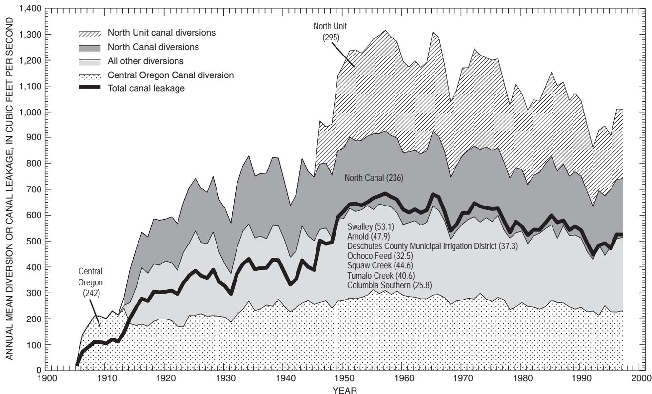
**Figure 10.** Annual canal diversions and estimated annual mean canal leakage in the upper Deschutes Basin, Oregon, 1905–97. (Mean annual discharge, in cubic feet per second, is shown in parentheses for the period of record for each diversion.)
