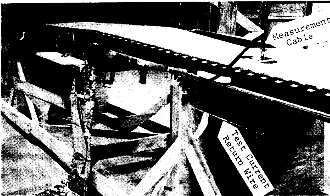
Figure 3.34 - Lab Setup for Bond Line and Fuel Probe Voltage Measurements in gr/E Wing.
