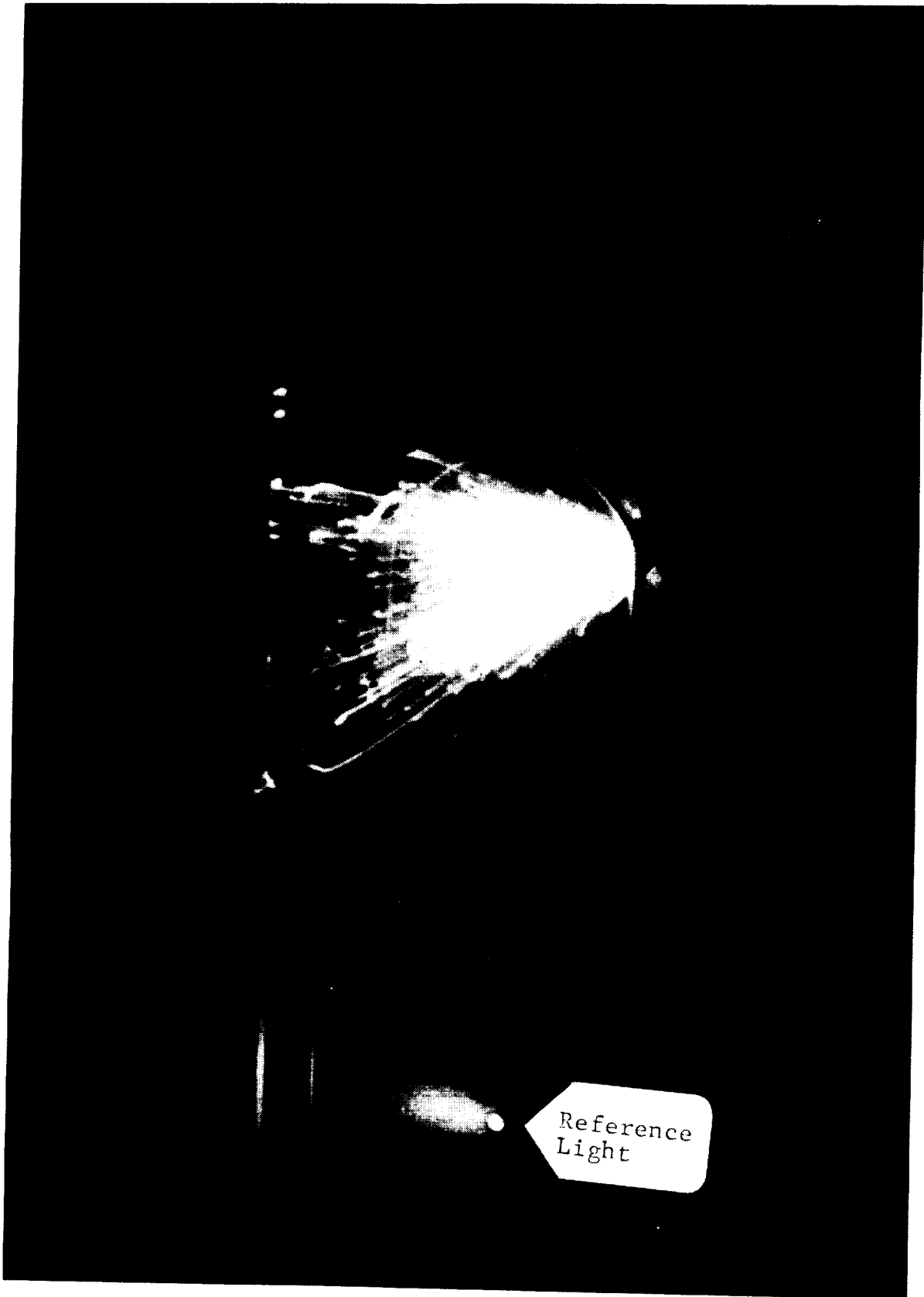
Figure 2.29 - Transfer of Current from Access Door to Splice Plate.
