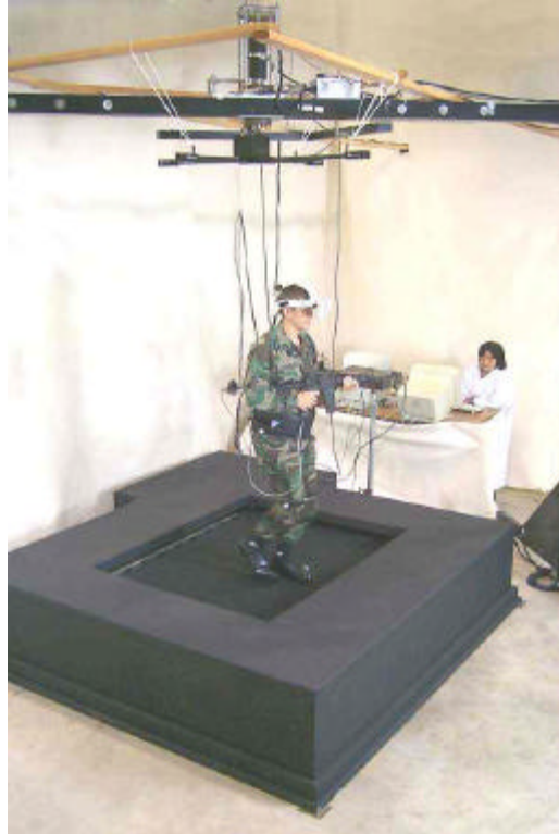
Figure 5. The Omni-Directional Treadmill with the sound enclosure.
