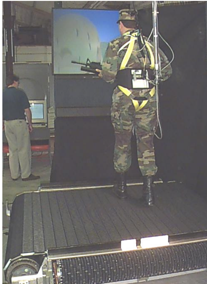
Figure 2. The original Omni-Directional Treadmill (approximately 1997).
