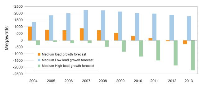
Since 2000, over 4,500 megawatts of generating capacity has been built in the Northwest. This, combined with the loss of load shown in the demand forecast graph, has led to a surplus of generation. The bars in this graph show the amount of generation in excess of load for three demand forecasts. The graph indicates that under the most likely range of load growth, new generating resources are unlikely to be needed until the end of the decade.
