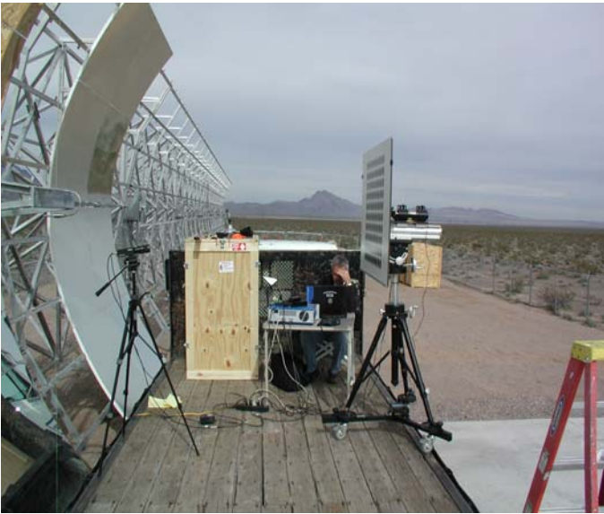
Figure 3. The VSHOT test setup at the Solargenix Test Loop in Boulder City, Nevada.
