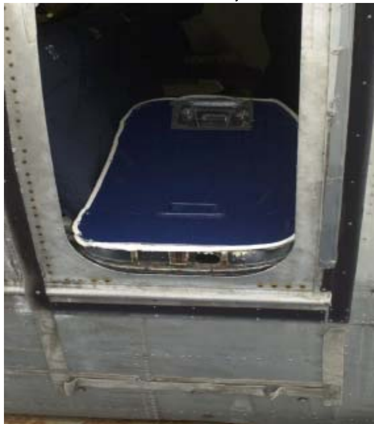
Figure 30 Slide to Exit Formed by Hatch
