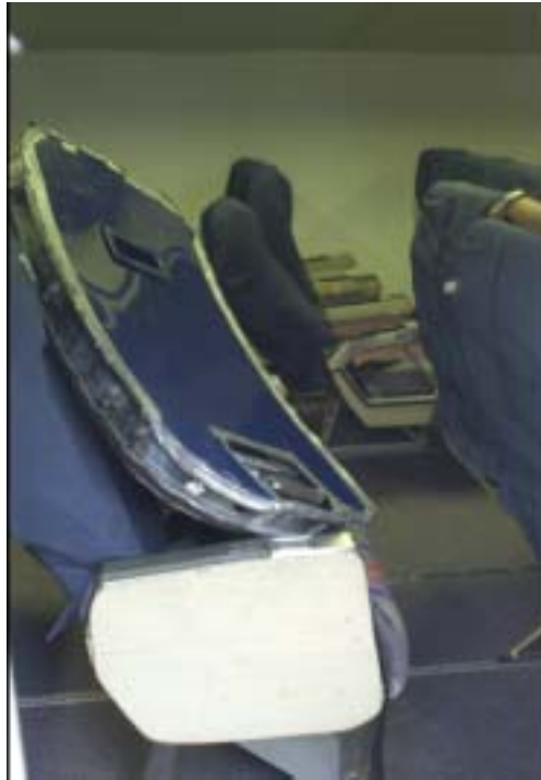
Figure 5 Typical Inside Hatch Disposal Location
