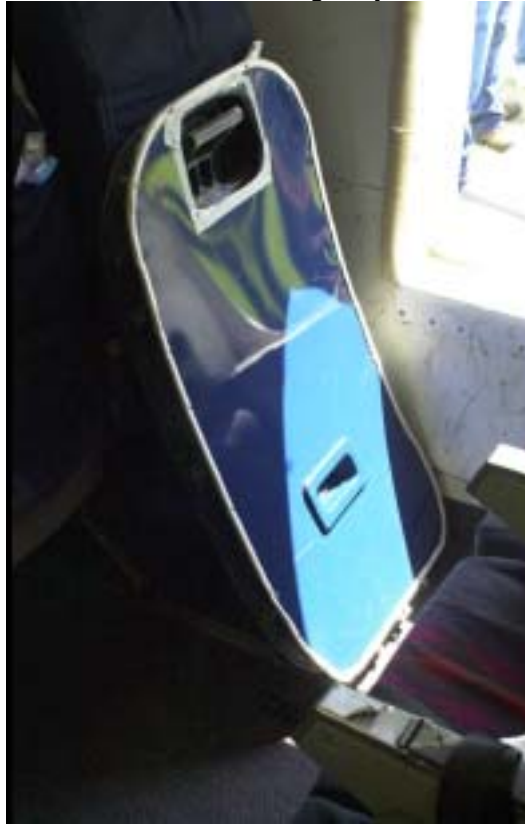
Figure 18 Hatch Stood on Passageway Floor
