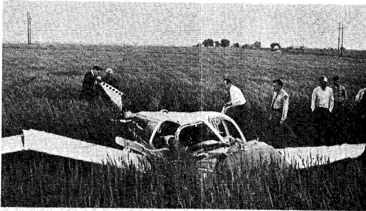
A. Aircraft crashed flat in a tall wheat field. Note wheat all around aircraft is undisturbed.
