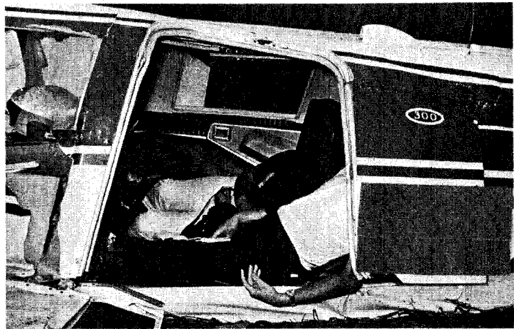
G, H & I All occupants have seat belts fastened, appear to be sitting on the ground, & died from severe internal injuries produced by vertical forces.
