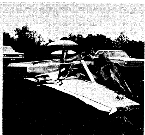
B. Forward motion of the aircraft was stopped when motor plowed under a large flat rock.
