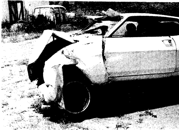
FIGURE 30. Side view of vehicle showing crushing of front end during deceleration.
