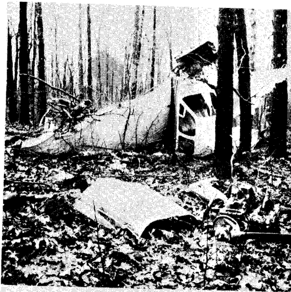
A. Wreckage of Beech Bonanza. Note that the tail, wings, & motor are torn away, but the cabin is intact.
