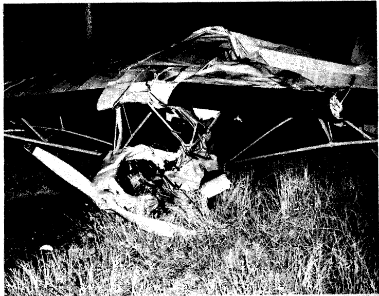
B. Front view showing tubular framework of this aircraft prevented cabin collapse.
