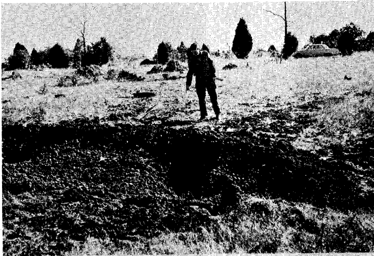
A. Crater formed by aircraft impact 38' long, 12' wide, & 4' deep.
