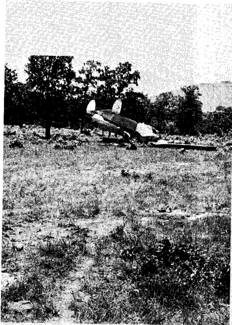
A. Distant view of resting aircraft & part of its 114-foot skid mark.
