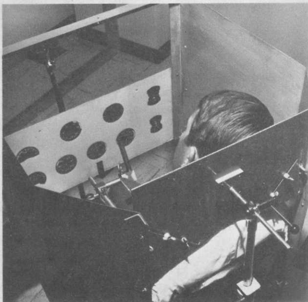
FIGURE 1. Modifications of a rotating device to control head movements and to introduce an aviation-related visual environment. The rod extending upward from the foot rest terminates in a plastic panel which contains three tiny lights (a red and a green "wing-tip" light and a flashing red "beacon") simulating an approaching aircraft. Upper left: rotation device without the "cabin" attachment (the chin rest depicted here is used for research rather than demonstration purposes). Upper right: the major section of the "cabin" has been bolted to the back of the head rest; its base is further supported by small metal extensions projecting outward from the arms of the chair. Lower left: the instrument panel is added to the "cabin" by means of four wing-nuts. Lower right: interior view of the "cabin" with a subject's head tilted to the right; the lights of the approaching aircraft were viewed through the "window" of the "cabin." The interior of the "cabin" was coated with luminous paint.
