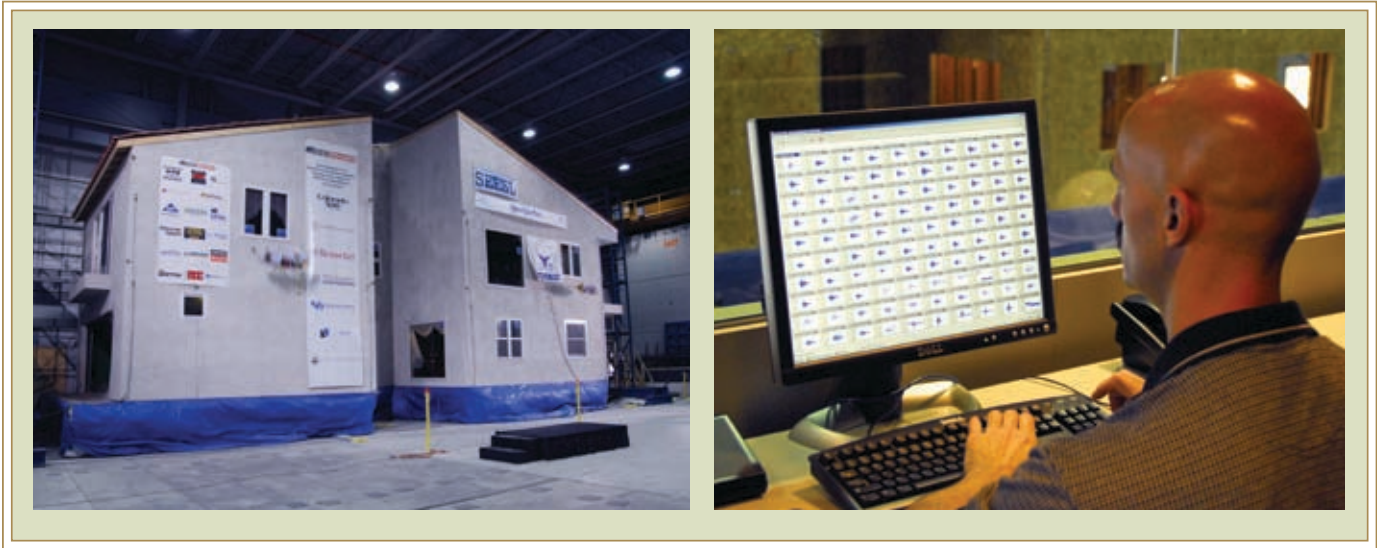
The NEES@buffalo shake table recreates movements of the forces generated by an actual earthquake. NEES allows earthquake engineers and students located at different institutions to share resources, collaborate on testing, and exploit new computational technologies.
