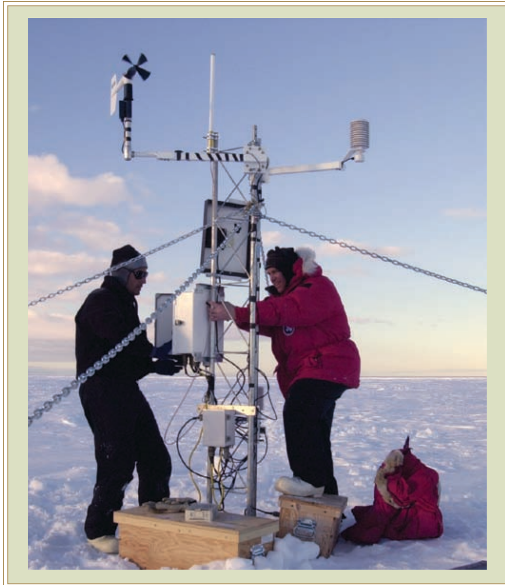
Researchers upgrade the software of an automated weather station that transmits data to help track the iceberg's position in the Antarctic and reports on the microclimate of the ice surface.
