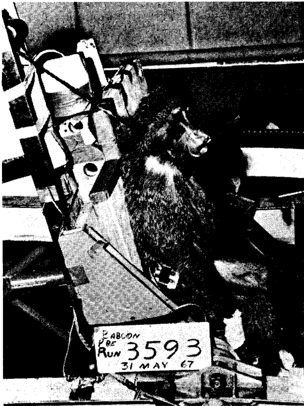
FIGURE 3. Yoke-type restraint with subject in place prior to run. Shoulder belt angle is 45^\circ to inertia reel. Note position of right shoulder belt strain gauge.
