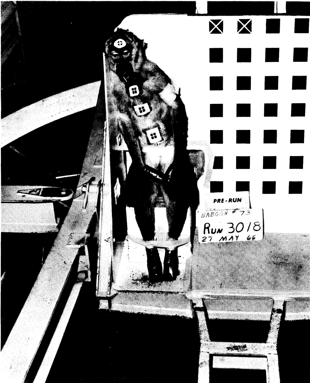
FIGURE 3. Baboon positioned in seat on omni-directional sled prior to impact run in lateral body position. Note photometric locators on animal and along portion of seat back.
