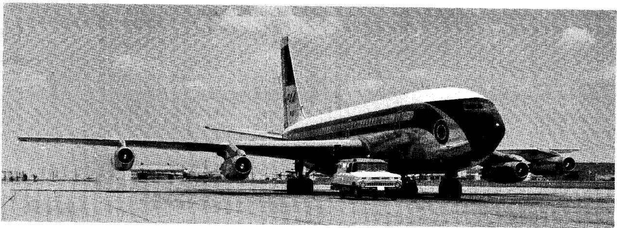
FIGURE 2. Boeing 720; a modern, "heavy" weight, sweptwing transport with four jet engines.
