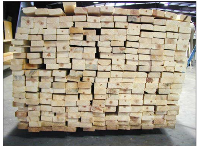
Figure 3—Standard and Better grade ponderosa pine lumber. Approximately 36% of pieces have pith-associated wood.
