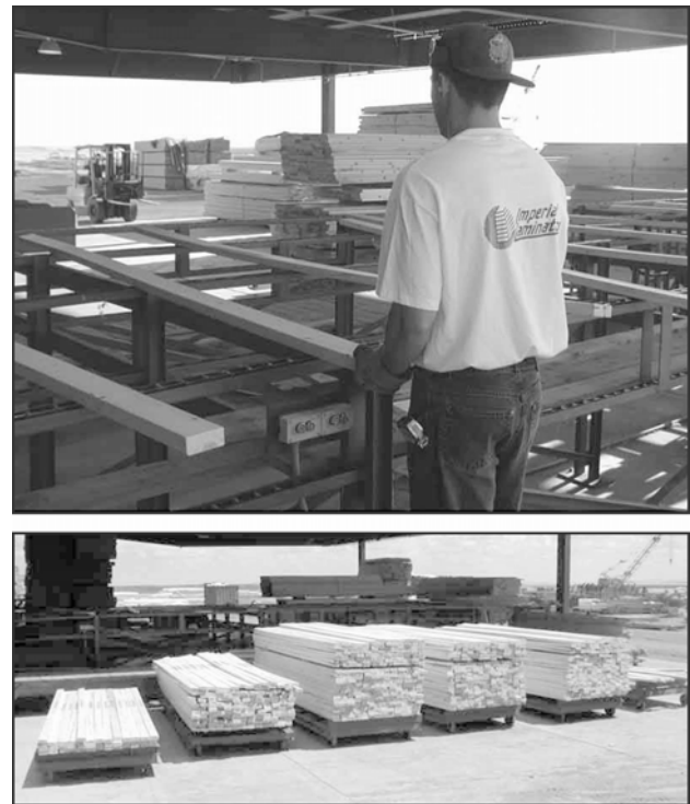
Figure 5—Grading of lumber: (top) visual grading of lumber after exiting CLT machine; (bottom) bundles of lumber sorted by MOE and visual lumber grade.
