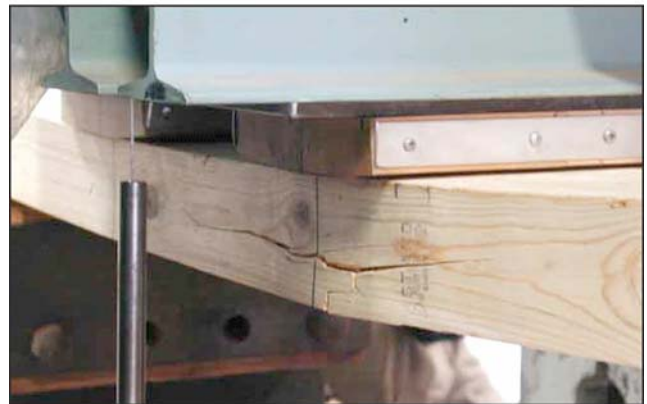
Figure 11—Testing of 13-lamination glulam beam: (top) flatwise bending test; (bottom) LVDT placement for measuring center-span deflection.
