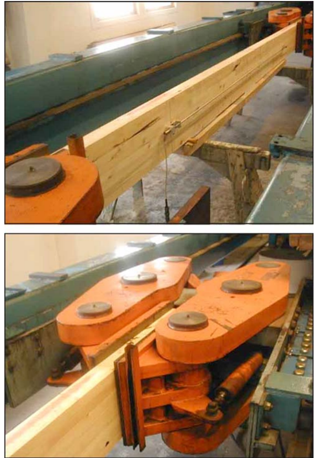
Figure 13—Testing of 8-lamination glulam beam: (top) tension test; (bottom) close-up of tension grips.
