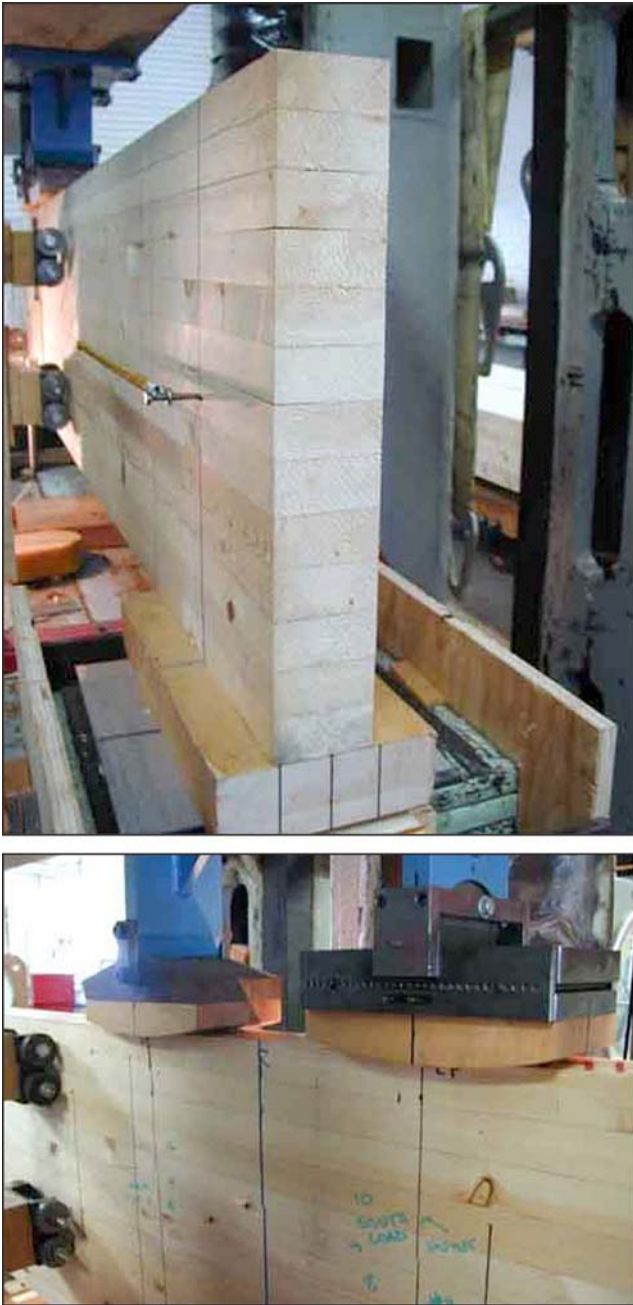
Figure 12—Glulam beam shear tests: (top) end view of support block, stringline for measuring deflection, and lateral supports; (bottom) close-up of load points and radiused contact blocks.
