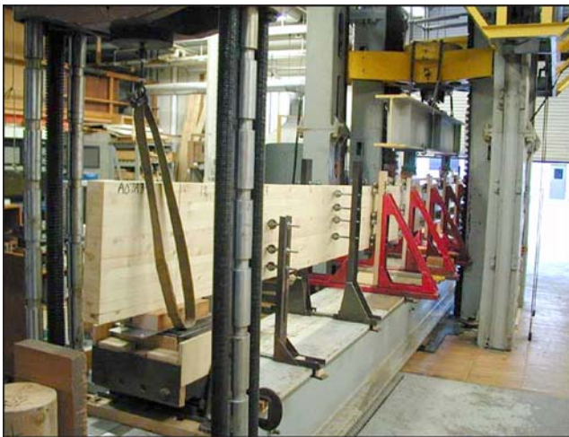
Figure 10—Edgewise bending test of 13-lamination glulam beam.
