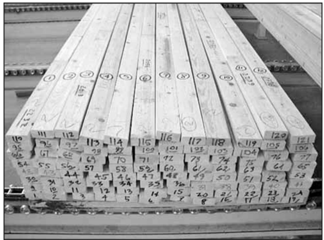
Figure 7—Dry stacking of finger-jointed laminating lumber. Note lumber, lamination, and beam identification numbers.
