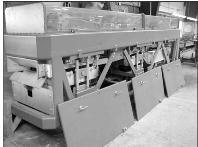
Figure 4—Continuous lumber tester used to test lumber for MOE. Panels removed to show rollers.
