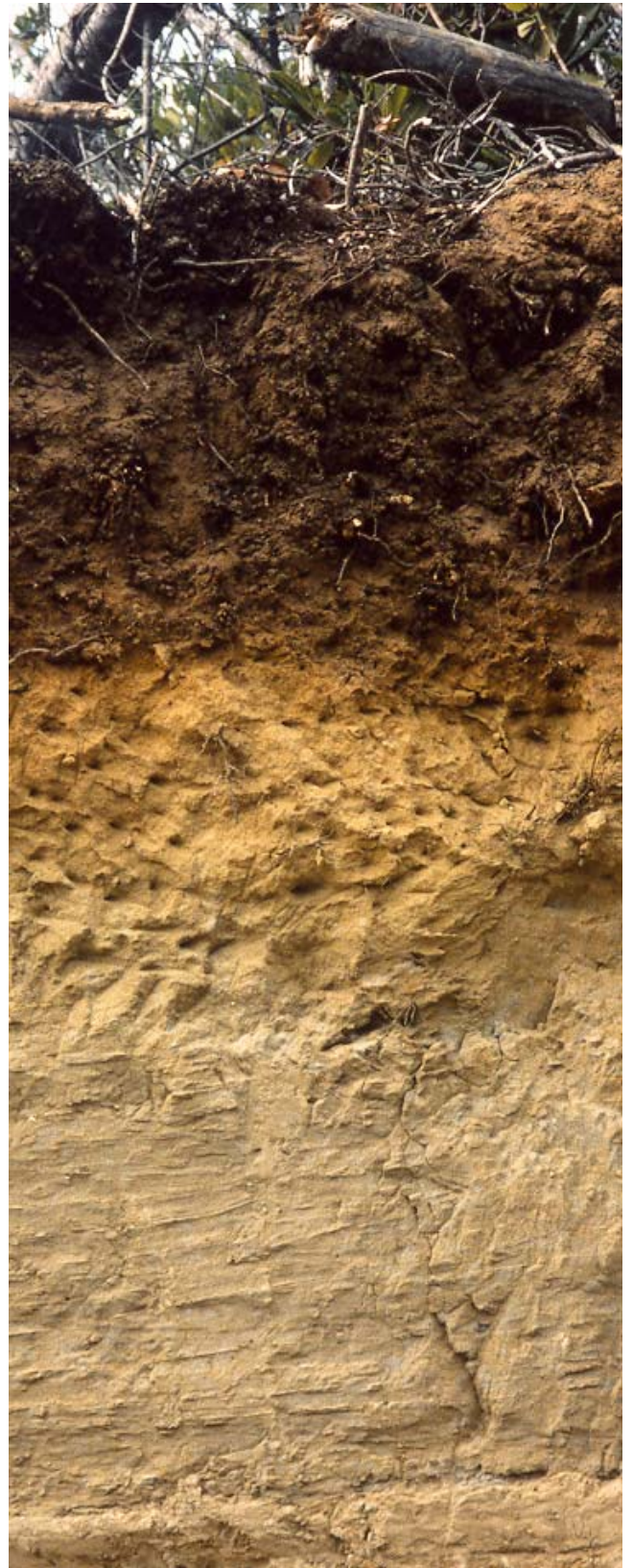
Figure 19.—Profile of a Bullards sandy loam showing the very dark grayish brown surface horizon over the dark yellowish brown and yellowish brown spodic horizon.
