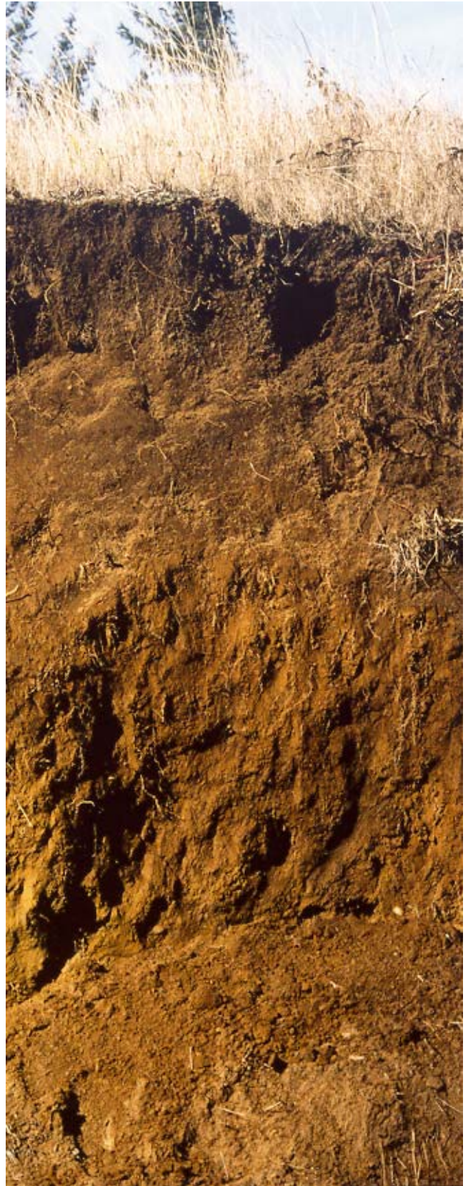
Figure 25.—Profile of a Quillamook silt loam showing the thick, dark-colored surface horizon.
