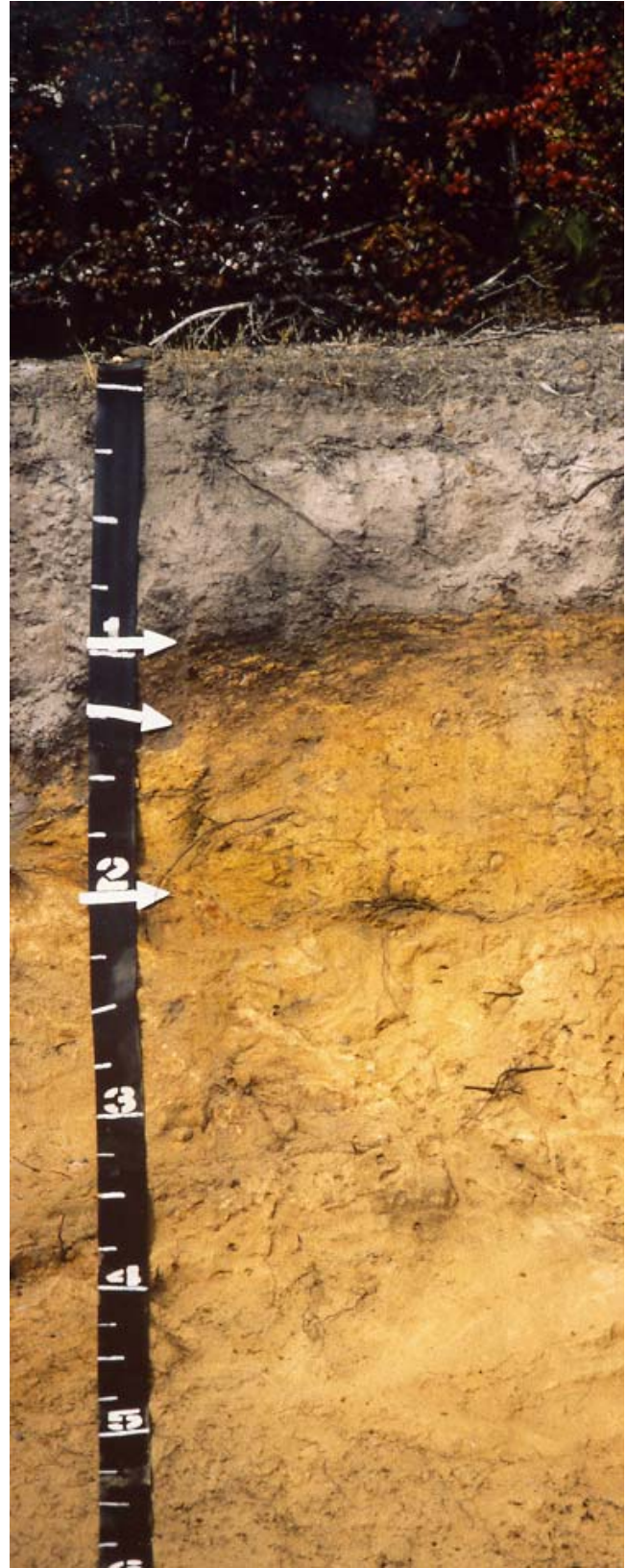
Figure 21.—Profile of a Cashner loam. A Bh horizon is at a depth of 12 inches, and it is underlain by a cemented spodic horizon.
