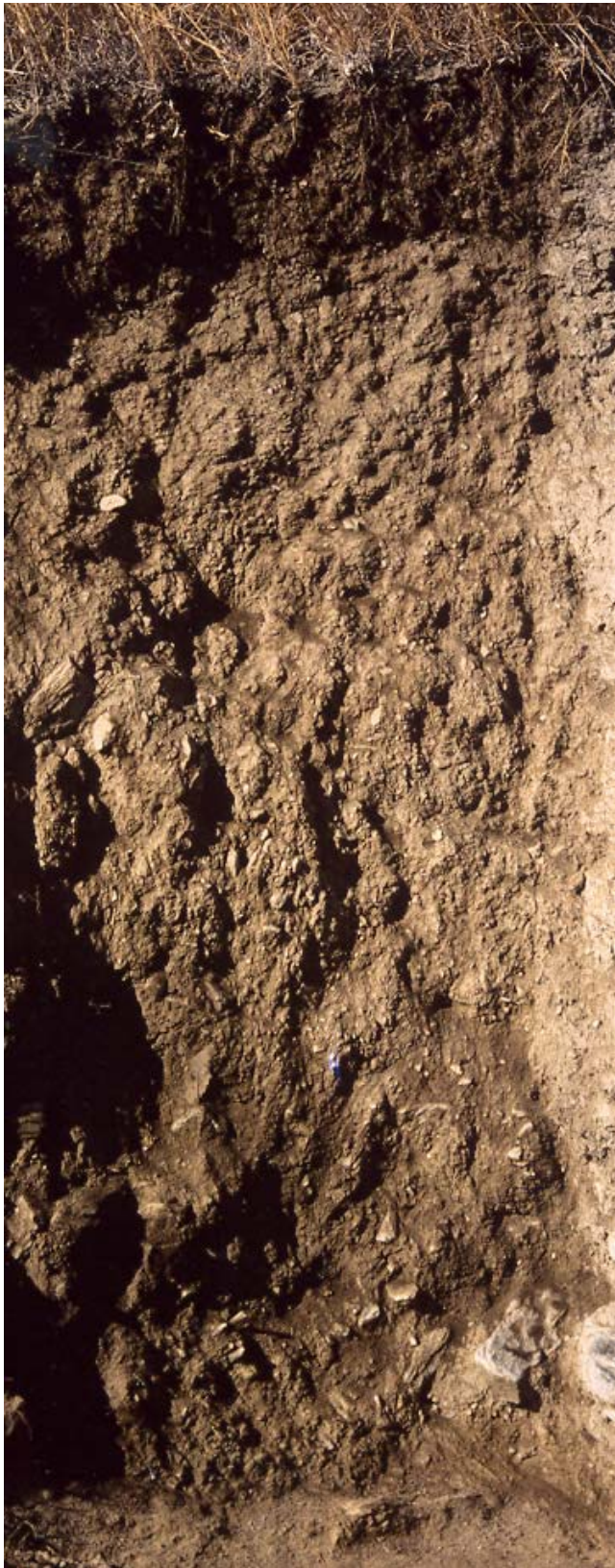
Figure 18.—Profile of an Agness channery silt loam showing the linear, platy rock fragments throughout.
