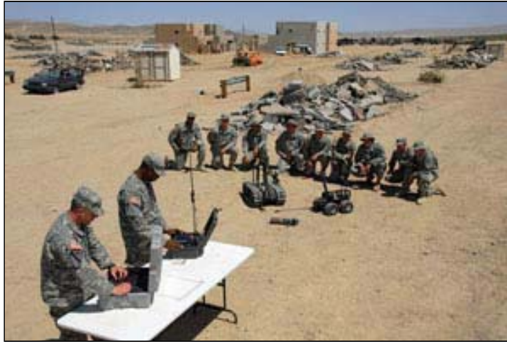
Soldiers learn to drive the Talon IIIB explosive ordnance disposal robot and the MarcBot while searching for IEDs hidden in the rubble behind them at the National Training Center.
