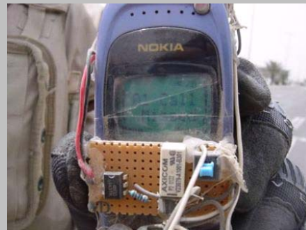
An EOD expert holds a cell phone IED triggering device that malfunctioned.
