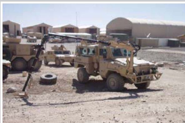
JIEDDO has funded a 26-foot mechanical interrogator arm that allows stand-off probing of suspected IEDs.
