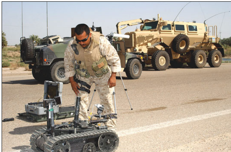
A Marine of the 15th Marine Expeditionary Unit assigned to Explosive Ordnance Team 8 prepares a Talon II remote-controlled robot to go down range and investigate a possible IED along the shoulder of a busy highway in southern Iraq.
