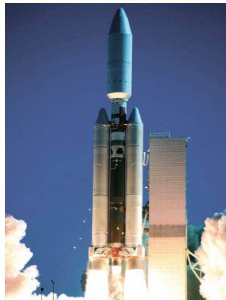
The Titan IVB is the largest unmanned space booster used by the Air Force.
