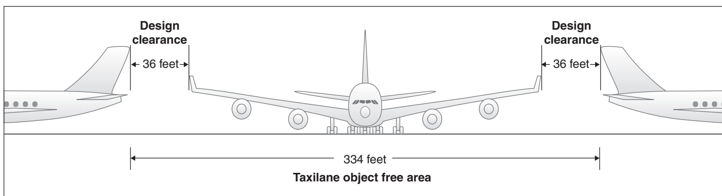
Figure 6: The Taxilane Object Free Area Requirement for the A380
