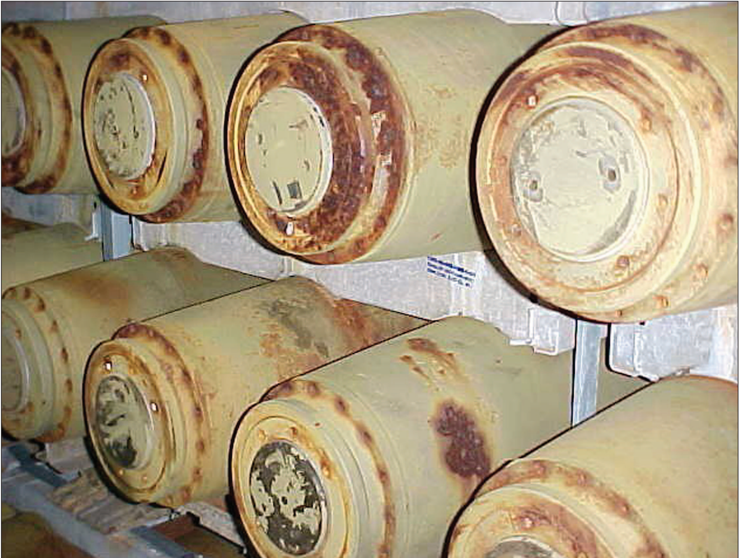
Figure 4: Corroded 500-Pound Bombs at Andersen Air Force Base, Guam
