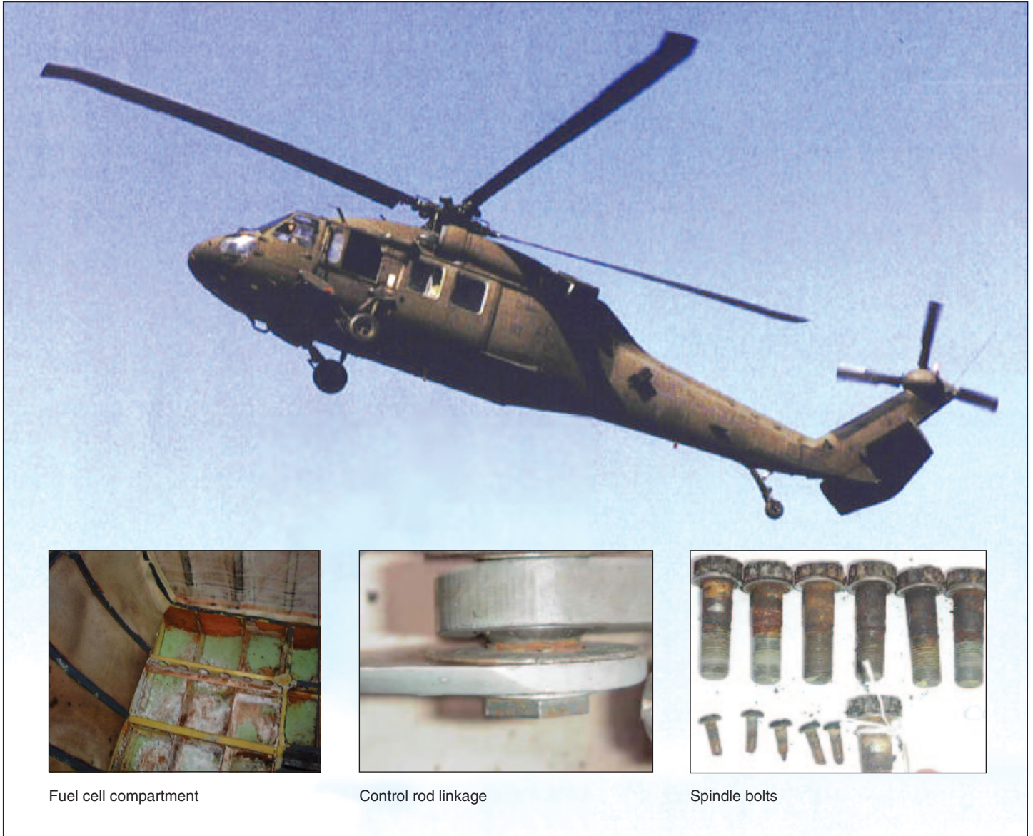
Figure 3: Corrosion on Army UH-60L Black Hawk Helicopter
