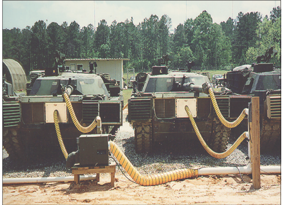
Figure 7: Army National Guard Controlled Humidity Preservation
