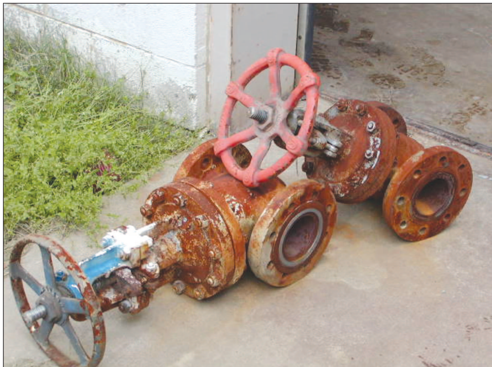
Figure 12: Corroded Air-Conditioning Valves at Quantico Marine Corps Base, Virginia
