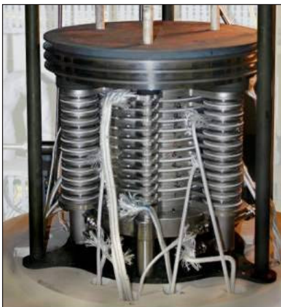
Fuel Cells: General Electric (GE) prototype for radial stacked planar solid oxide fuel cells.
