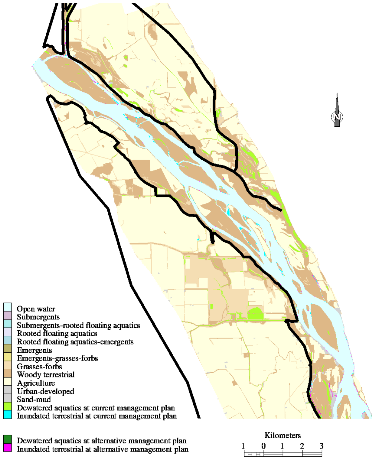
Figure 21. Comparison between water level management plan (Plan 2) and the present plan (Plan 1) at 19,000 cfs for land cover classes in the northern portion of Pool 25.
