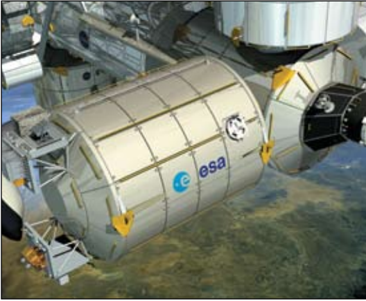
Columbus is a multifunctional pressurized laboratory to carry out experiments in materials science, fluid physics, and biosciences, as well as to perform technological applications.
