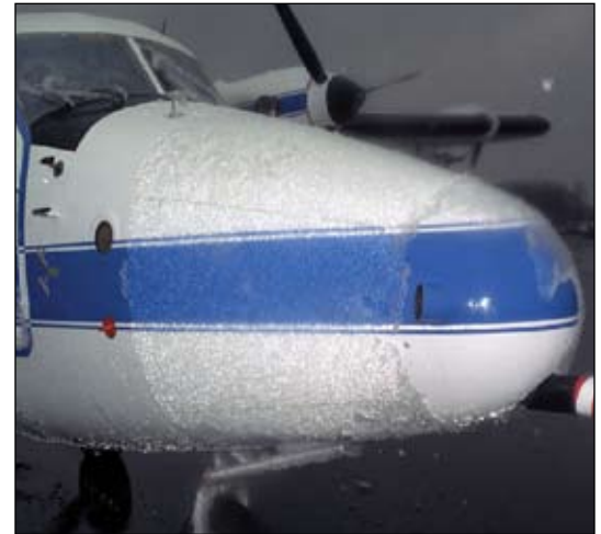
Post-flight image shows ice contamination as a result of encountering SLD conditions near Parkersburg, West Virginia.
