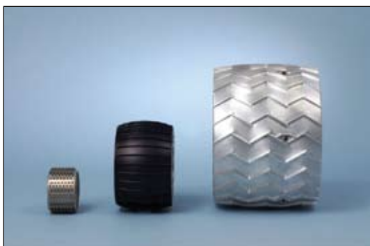
This image indicates the growing wheel size between the various Mars explorers: Pathfinder, Mars Exploration Rover, and MSL.
