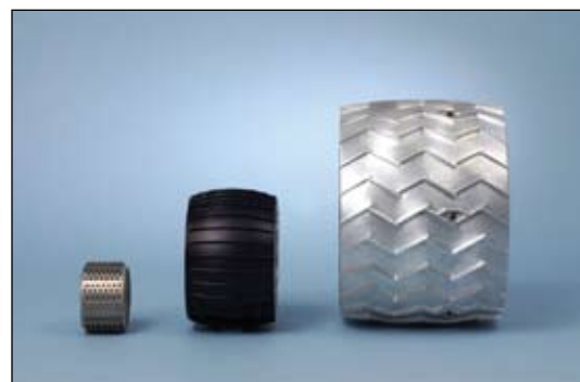
This image indicates the growing wheel size between the various Mars explorers: Pathfinder (left), Mars Exploration Rover, and MSL.
