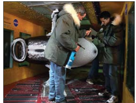
Technicians taking measurement of ice accretions after an icing test at Glenn Research Center.
