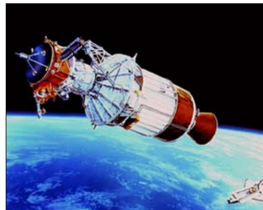
Depicted here is an artist concept of Ulysses after deployment from the Space Shuttle cargo bay. Ulysses is a combined upper-stage vehicle, consisting of an Inertial Upper Stage and a Payload Assist Module, both of which propelled Ulysses away from the Earth toward Jupiter.
