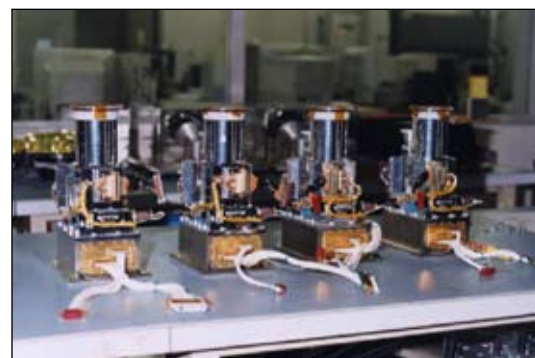
The four XIS instruments before their installation into the Suzaku spacecraft
