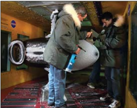
Technicians taking measurement of ice accretions after an icing test at Glenn Research Center.
