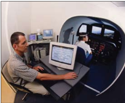
The Intelligent Spacecraft Interface Systems Lab contains a reconfigurable cockpit simulator, which is used to gather human performance data for current and future vehicle display designs.
