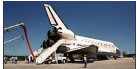
Landing convoys such as these at KSC would provide support to the Space Shuttle crew in the event of a landing at a TAL site.
