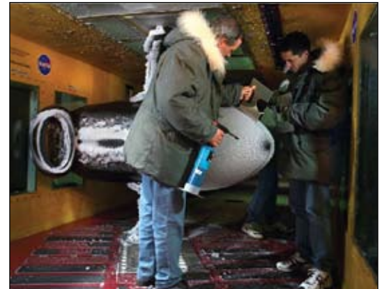
Technicians measure ice accretions after an icing test at Glenn Research Center.
