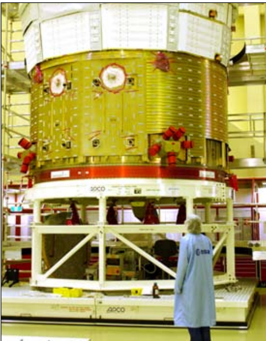
The ATV is an autonomous logistical resupply vehicle designed to dock to the ISS and provide the crew with dry cargo, atmospheric gas, water, and propellant.
