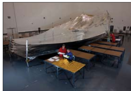
Designed to block solar light and keep the JWST Observatory operating at cryogenic temperature, the five-layer sunshield consists of thin membranes made from a polymer-based film and supporting equipment such as spreader bars, booms, cabling, and containment shells.
