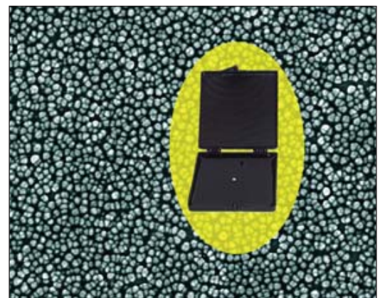
Figure 2. The RM 8091 Sharpness Reference Material.
