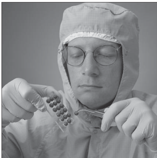
Christopher Holloway tests a composite medium consisting of insulating magneto-dielectric spherical particles embedded in a background matrix for double negative index behavior. © Geoffrey Wheeler
