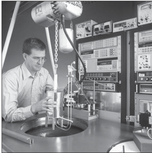
Jim McLean prepares to lower a waveguide microwave calorimeter into a water bath. © Geoffrey Wheeler
