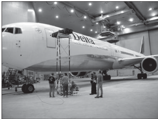
Evaluation of a commercial aircraft using a portable NIST time-domain measurement system.
