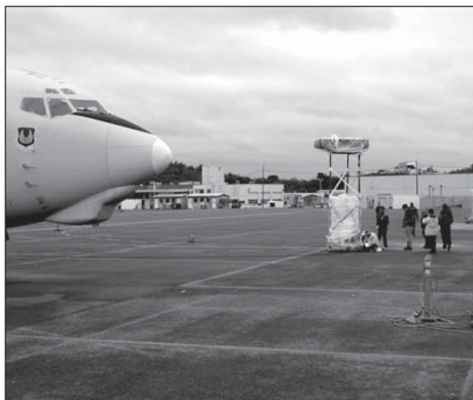
Evaluation of a U.S. Air Force early-warning aircraft using a portable NIST time-domain measurement system.
