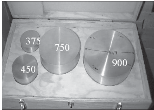
The basic cylinder set used to calibrate static RCS measurement systems in the frequency range of 2 to 18 gigahertz. The cylinders are made of aluminum, and are manufactured to a tolerance of \pm 0.127 millimeter.
