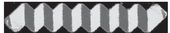
Micrograph of a zig-zag magneto-resistive element obtained by use of a scanning electron microscope with polarization analysis (SEMPA). With respect to the long axis of the sensor (the axis of current), light gray indicates magnetization at an angle of +45 degrees, dark gray at an angle of -45 degrees. The magnetic domain patterns were also accurately modeled with NIST's Object Oriented MicroMagnetic Framework (OOMMF).
