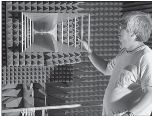
Doug Tamura aligns a dual ridge horn for measurements.
