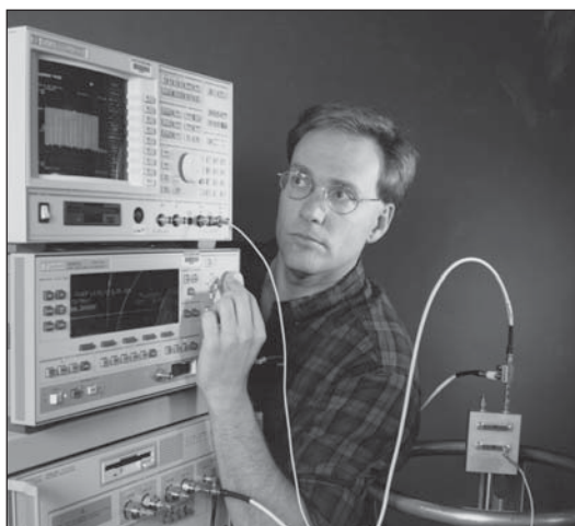
Sam Benz optimizes the operating margins for the Josephson arbitrary-waveform synthesizer.
