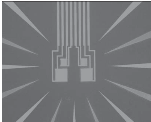
Array of four Transition Edge Sensor (TES) single-photon detectors. The larger squares are 50 \mu\text{m} on a side and the smaller ones are 25 \mu\text{m} . The arrows are for alignment.
