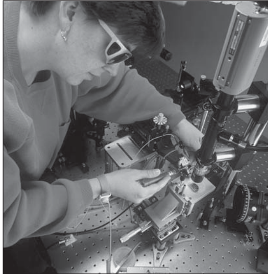
The electro-optic measurement system, shown here being operated by Tracy Clement, measures an electrical pulse on a LiTaO 3 wafer. De-embedding techniques are then used to determine the voltage generated by the photodiode being tested at its coaxial output connector. (© Geoffrey Wheeler)
