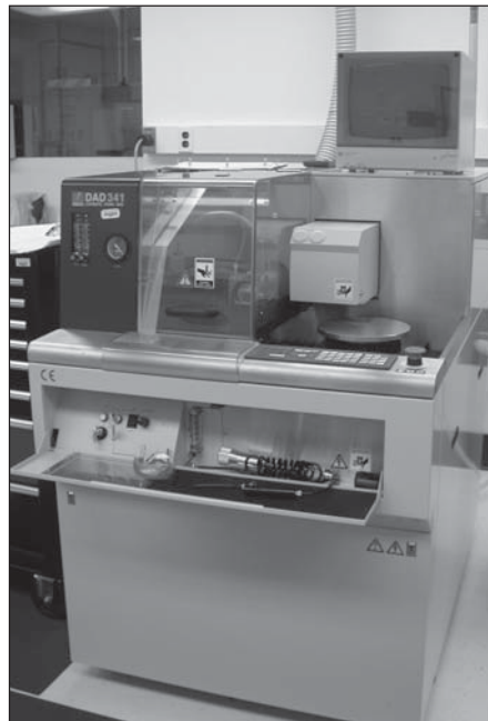
Automatic 8" wafer dicing saw.
