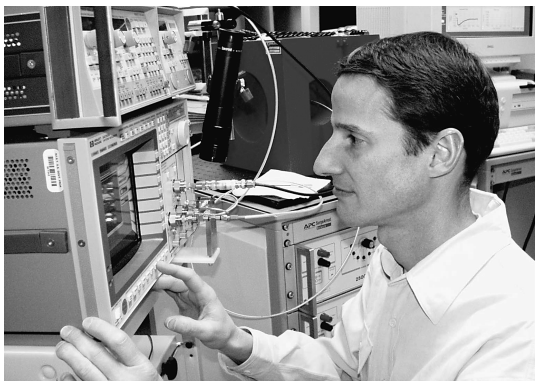
Electronics engineer Tony Kos operating the pulsed inductive microwave magnetometer (PIMM).
