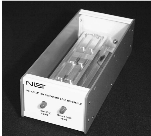
Measurement Assurance Program artifact exhibits stable polarization-dependent loss, certified as a function of wavelength.
