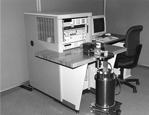
**Noise figure radiometer and cryogenic standard**
