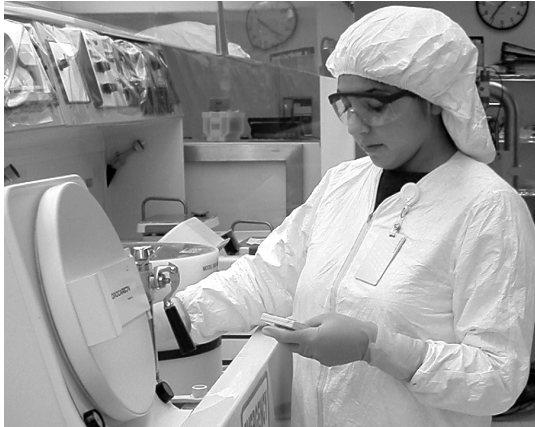
Christine Murabito using a hot plate to do a post-exposure bake during the photo-lithography process.
