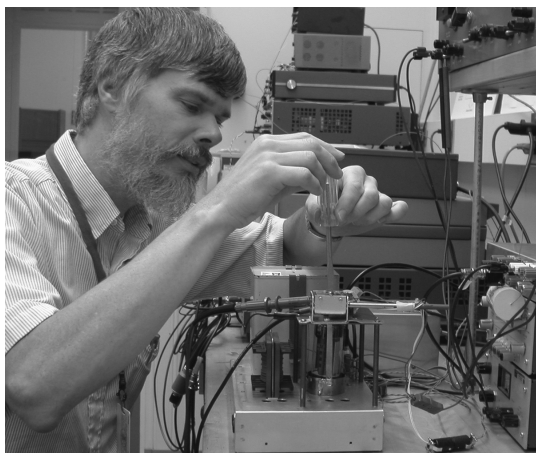
David Berning measuring silicon carbide diodes using NIST-developed, specialized equipment, not commercially available.
