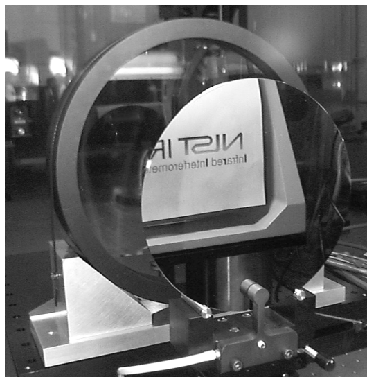
CURRENT WAFER HOLDING MECHANISM (VIEWED FROM THE WAFER BACK SIDE). THE SMALL VACUUM ORIFICE IS SEEN AT THE LOWER EDGE OF THE 200 MM WAFER. BEYOND THE WAFER IS AN F/6 300 MM COLLIMATOR.
