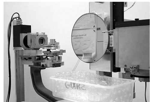
A HIGH RESOLUTION X-RAY REFLECTOMETRY SYSTEM WAS DESIGNED AND OPTIMIZED FOR THE ROUTINE ANALYSIS OF COMPLEX THIN FILM AND MULTILAYER STRUCTURES THAT ARE OF INTEREST TO THE SEMICONDUCTOR INDUSTRY
