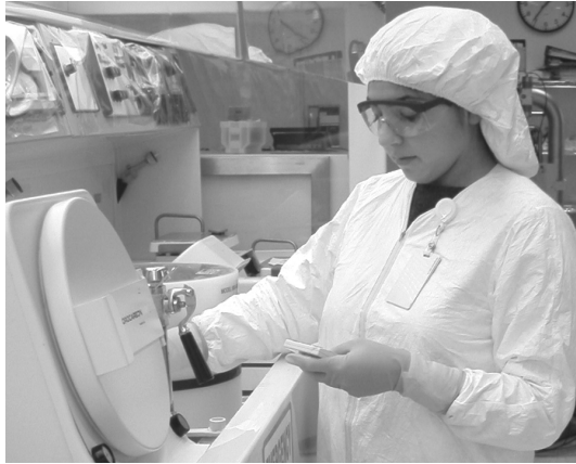
CHRISTINE MURABITO USING HOT PLATE TO DO A POST-EXPOSURE BAKE DURING THE PHOTO-LITHOGRAPHY PROCESS.
