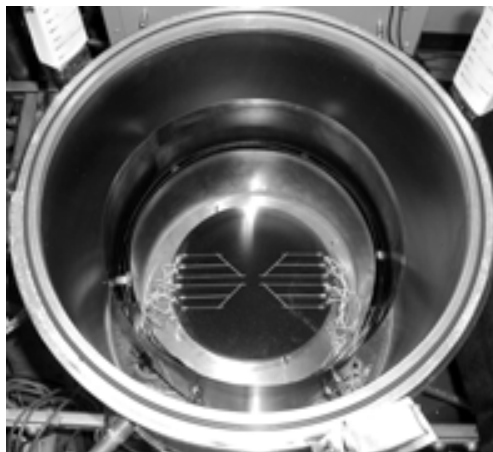
NIST TFTC TEST WAFER IN THE ISMT-UT TEST BED BEING DEVELOPED TO QUALIFY COMMERCIAL CONTACT AND RADIATION THERMOMETRY INSTRUMENTATION, AND ESTABLISH UNCERTAINTIES IN THEIR TRACEABILITY TO THE ITS-90.
