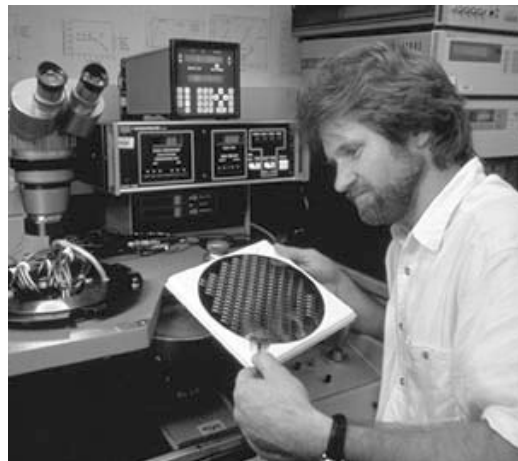
Dr. John Suehle preparing to load a sample on wafer prober
