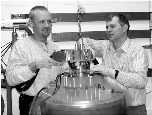
Ted Stauffer and Loren Goodrich lowering a test fixture into a critical current measurement cryostat. The cloud at the top of the cryostat results from the boiling cryogen.
