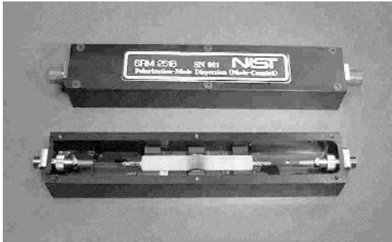
Polarization-mode dispersion (mode coupled) artifact (SRM 2518).
