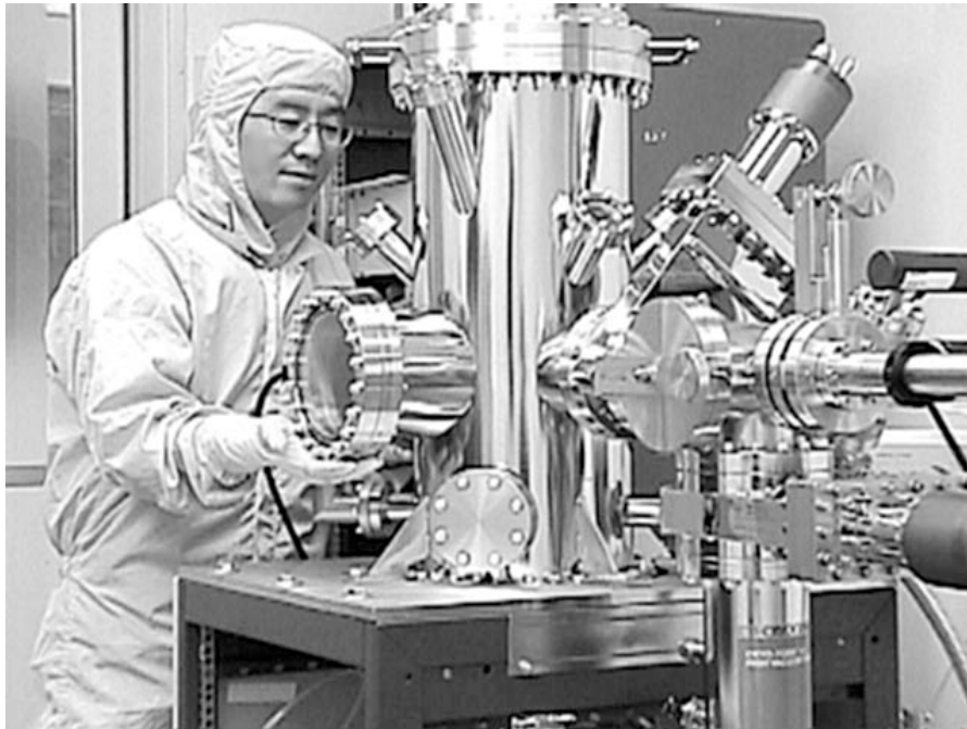
Post-doc Chulsoo Kim operating the chemically assisted ion-beam etching system for photonic crystal fabrication
