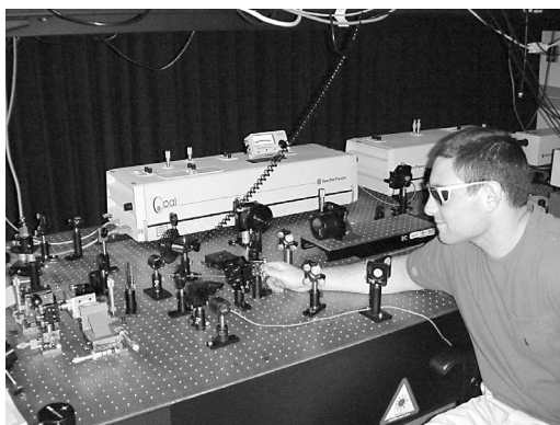
Ultrafast measurement system with tunable wavelength for pump-probe characterization of compound semiconductor structures
