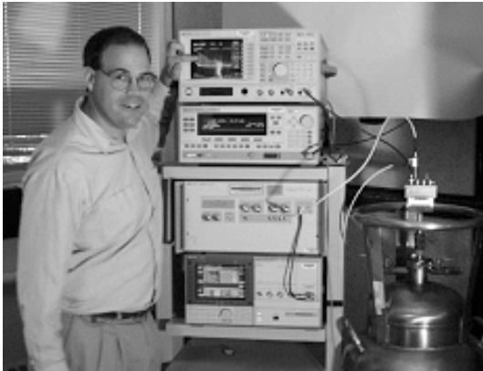
Paul Dresselhaus demonstrates a waveform synthesized with the Josephson arbitrary waveform generator.
