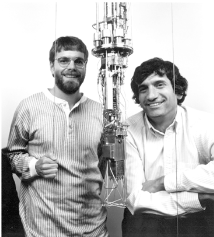
Mark Keller (left) and John Martinis with the dilution refrigerator used for the capacitance standard based on counting electrons.
