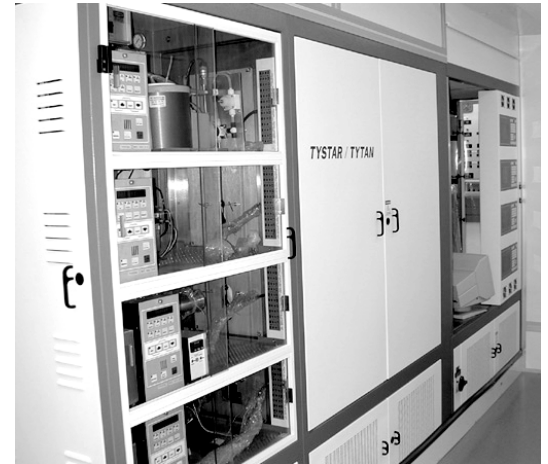
Computer-controlled research tube furnaces for growth of SiO 2 , Si 3 N 4 , and other CVD materials.
