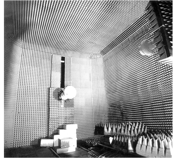
The NIST probe pattern range with the fixed probe located near the center of the photo and the moving probe located on the moving tower in the upper right of the photo.
