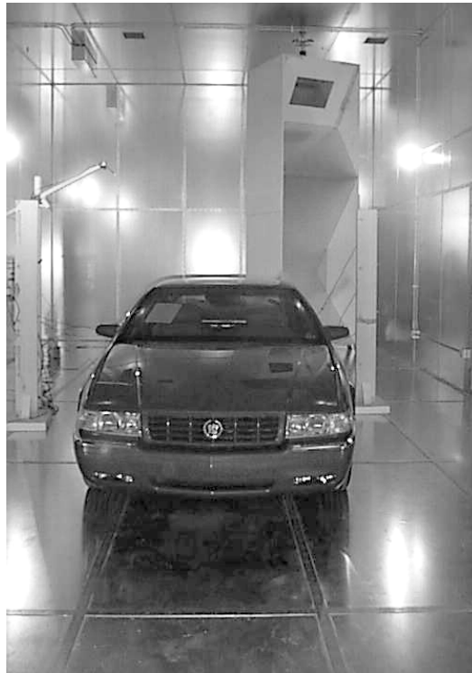
Evaluation of Reverberation Chamber techniques for vehicle EMC testing.
