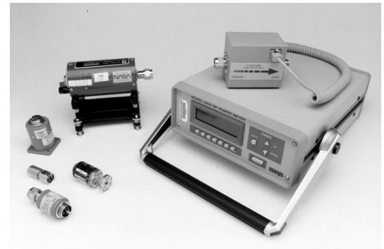
Microwave power meter and detectors
