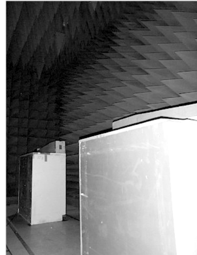
Absorber-lined chamber testing using NIST-developed time-domain fast-pulse measurement techniques.
