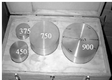
The basic cylinder set used to calibrate static RCS measurement systems in the frequency range of 2-18 GHz. The cylinders are made of aluminum, and are manufactured to a tolerance of \pm 0.0127 cm.
