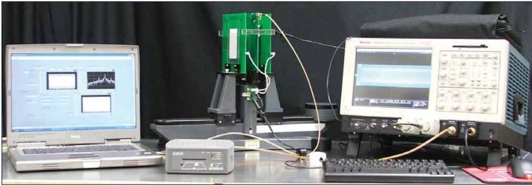
Setup for the 13.56 megahertz load modulation test, which is used to test the strength of the return signal from an RFID card.
