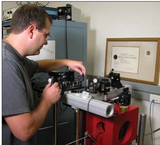
Time-resolved magneto-optic microprobe and pulsed inductive microwave magnetometer (PIMM) configured to simultaneously measure magnetization dynamics. Comparison of the two techniques permits quantitative determination of linewidth contribution due to spatial inhomogeneity of the gyromagnetic frequency.
