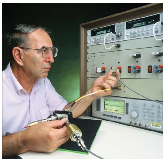
Calibration measurements on the direct comparison power system.
