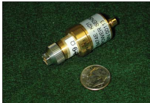
A 2.4 millimeter thin-film primary power transfer standard.
