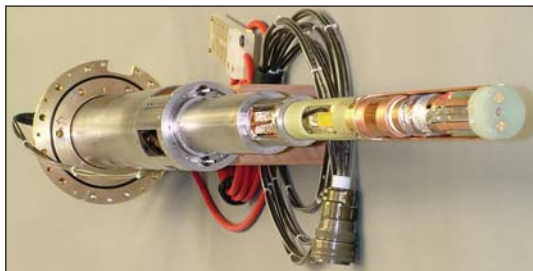
Probe for the measurement of the critical current of a superconductor wire as a function of temperature. The probe is inserted into the bore of a high field superconducting magnet.
