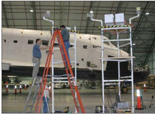
Division staff members perform field penetration tests on a NASA space orbiter.
