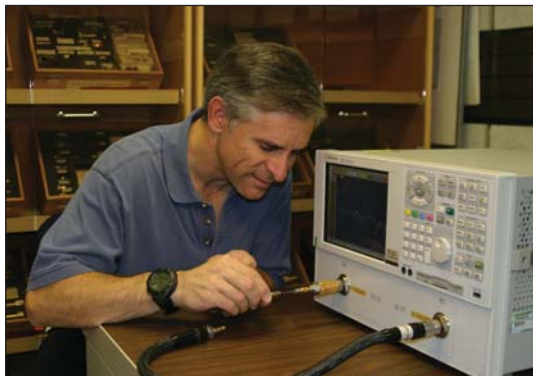
Setting up experimental vector network analyzer calibration using 1.5 millimeter airline standard.
