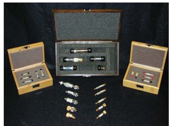
S-parameter measurement comparison kits for Type-N 7 millimeter, 3.5 millimeter, 2.92 millimeter and 2.4 millimeter coaxial connectors.
