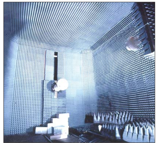
The NIST probe pattern range with the fixed probe located near the center of the photo and the moving probe located on the moving tower in the upper right.
