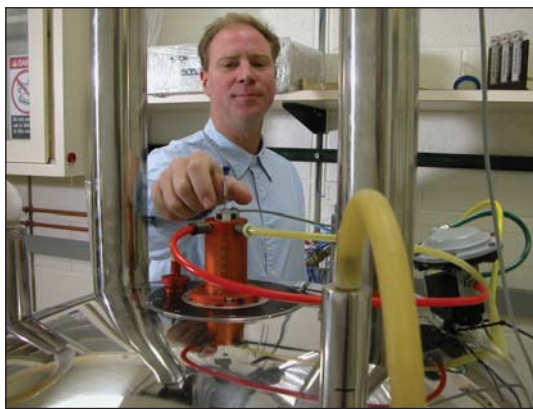
NMR system (7 teslas, 300 megahertz) for use in characterizing MRI contrast agents.
