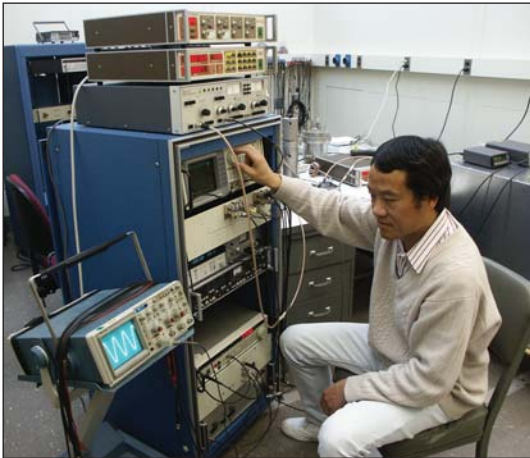
Yicheng Wang sets up an automated system for determining the frequency dependence of fused-silica capacitors.
