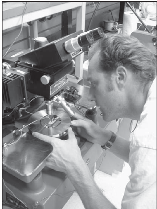
Ray Simmonds probes the resistance of Josephson junctions on a new wafer of quantum bits.
