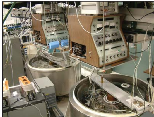
Two automated 1 ohm measurement systems allow precise customer tests and characterization studies.
