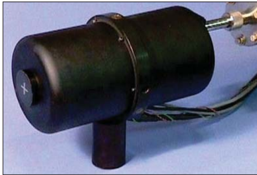
The C-Series Calorimeter, originally developed in the 1970s for use with cw lasers in the range from 50 \mu W to 1 W and 0.4 \mu m to 2 \mu m wavelength. Improved versions are in current use for calibrations.
