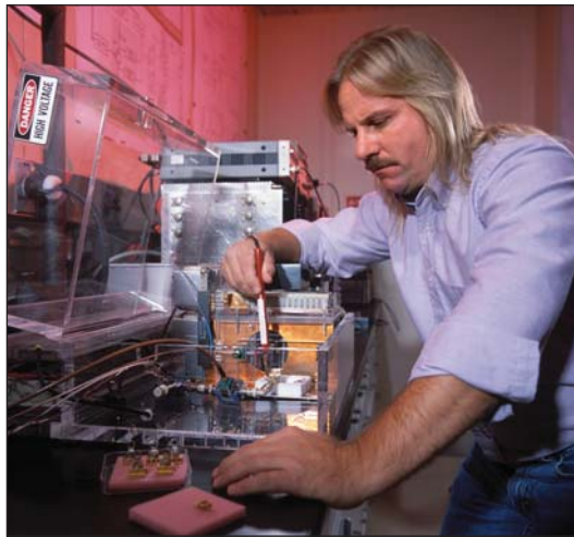
Allen Hefner, Jr., performs high-speed, high-voltage silicon carbide device characterization using NIST-developed, specialized equipment. Copyright Robert Rathe
