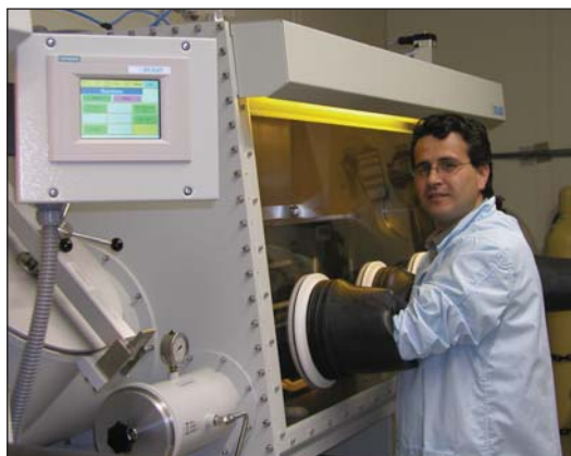
Modular glove box system in which organic electronic devices are fabricated and their initial current-voltage characteristics measured.
