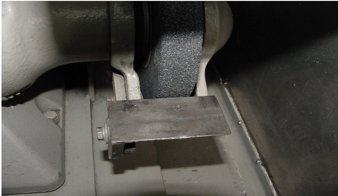
Tool Rest Correctly Adjusted
