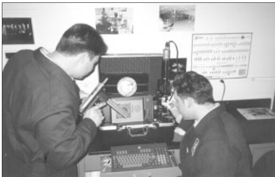
IBIS Specialists examine evidence being processed using the Rapid Brass Identification System technology.
