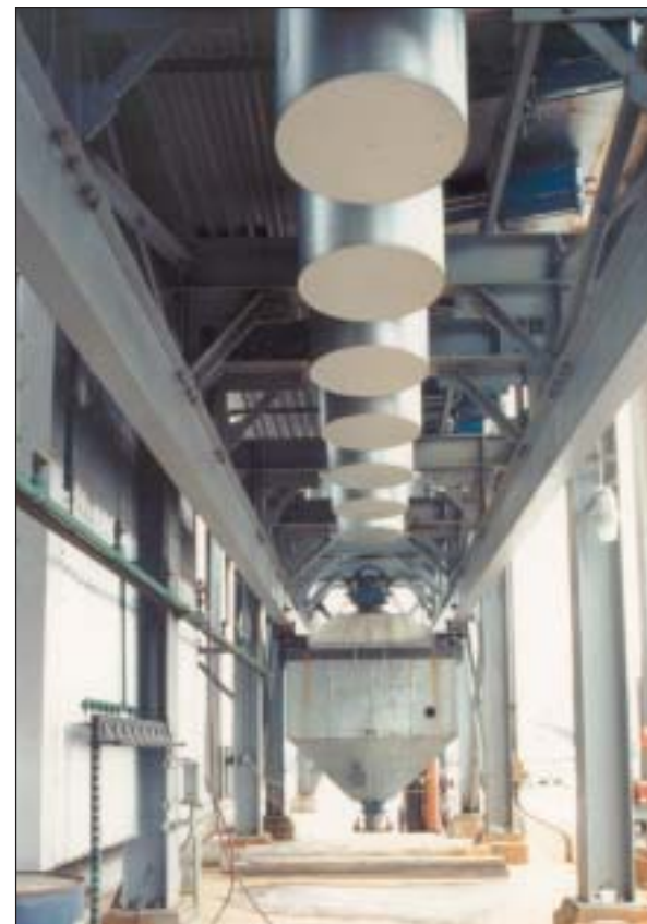
The bottom portion of the SO 2 converter reactor, with the catalyst dust collector hopper mounted on steel rails (center).
