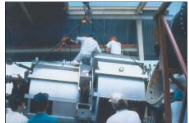
The TRW slagging combustor for the Healy Station.
