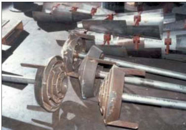
The S-Type burner impellers used in the LNCB ® design.
