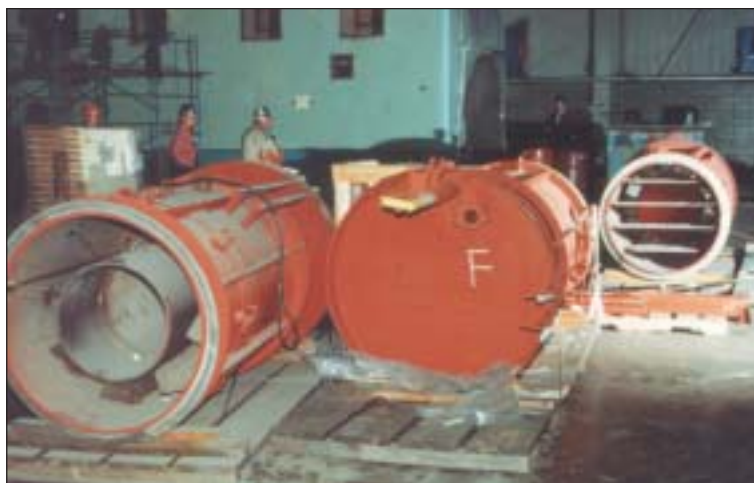
Cell burner AOFA connection with air control vanes open (right) laying next to cell burner housing showing primary air directional vanes and coal tube (left).
