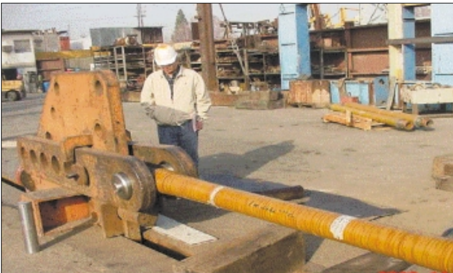
Figure 2: Tension Test on 1/3-Scale, 10-Foot Section of CDP
