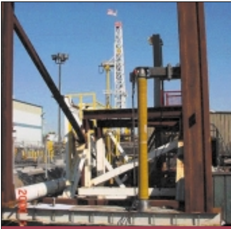
Figure 3: Torque Test on 1/3-Scale, 10-Foot Section of CDP
