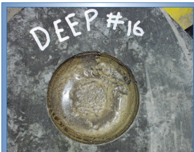
Figure 4. Mancos shale drilled with oil-based mud at high wellbore pressure
