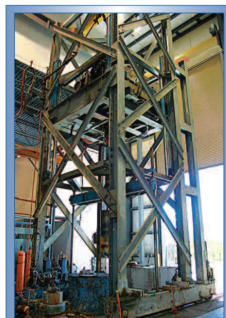
Figure 2. TerraTek full-scale drilling rig with high pressure wellbore simulator
