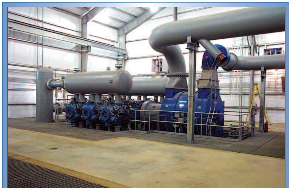
Figure 2. High-speed horsepower compressors are challenging pulsation control designers.
