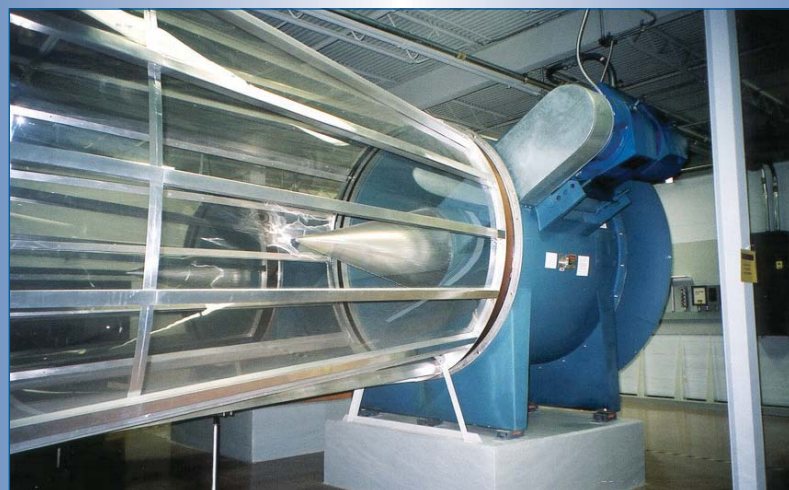
Figure 1. A fan for producing low-speed airflow is shown in the University of Arkansas's wind tunnel.
