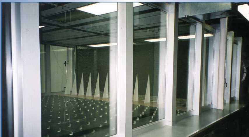
Figure 3. Fourteen Irwin spire-shaped structures generate turbulence in the low-speed wind tunnel.
