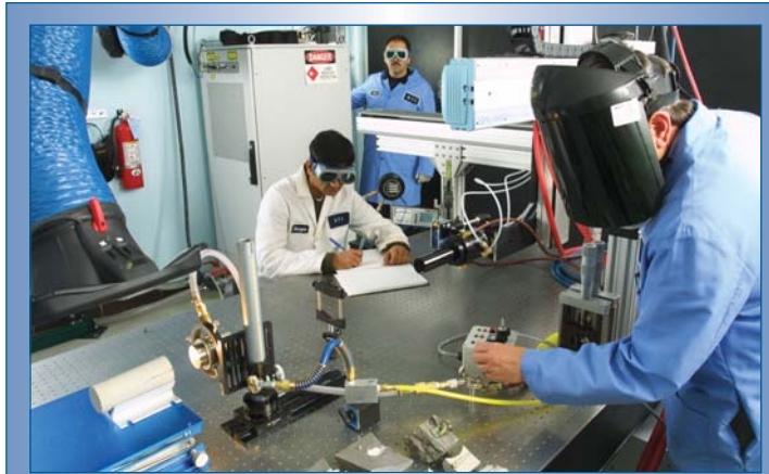
Figure 4. Researchers prepare to shoot a laser beam at the small cylindrical rock sample (lower left) in the Gas Technology Institute's new laser laboratory for exploration and production applications. The IPG Photonic 5-kW ytterbium fiber laser is in the vertical cabinet in the center background. (Photo courtesy of GTI)
