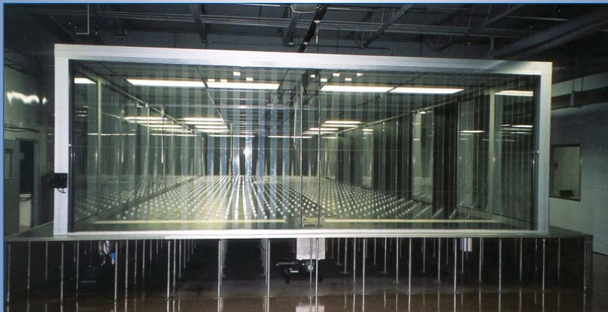
Figure 2. The working area of the low-speed wind tunnel comprises a space 7ft high, 20ft wide and 80ft long.
