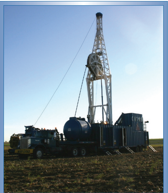
Figure 3. The hybrid microhole coiled tubing drilling rig developed by Advanced Drilling Technology/Coiled Tubing Solutions Inc. delivered 25% to 35% cost savings per well drilled compared with conventional rotary drilling equipment, drilling 3,000-ft Niobrara wells in as little as 19 hours.
