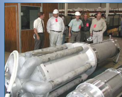
Figure 8. Ebara's liquefied natural gas pump in assembly.
