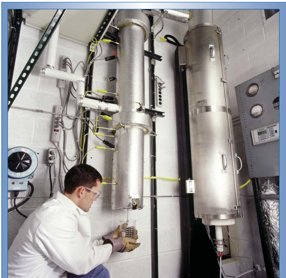
Figure 5. A bench-scale test of Gas Technology Institute's superadiabatic partial oxidation reactor facility.
