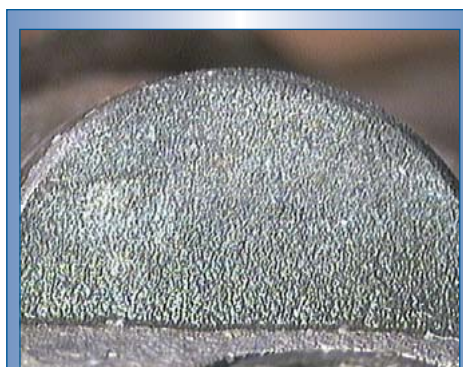
Figure 9. The above photo shows no impact damage to the improved thermally stable diamond cutter.
